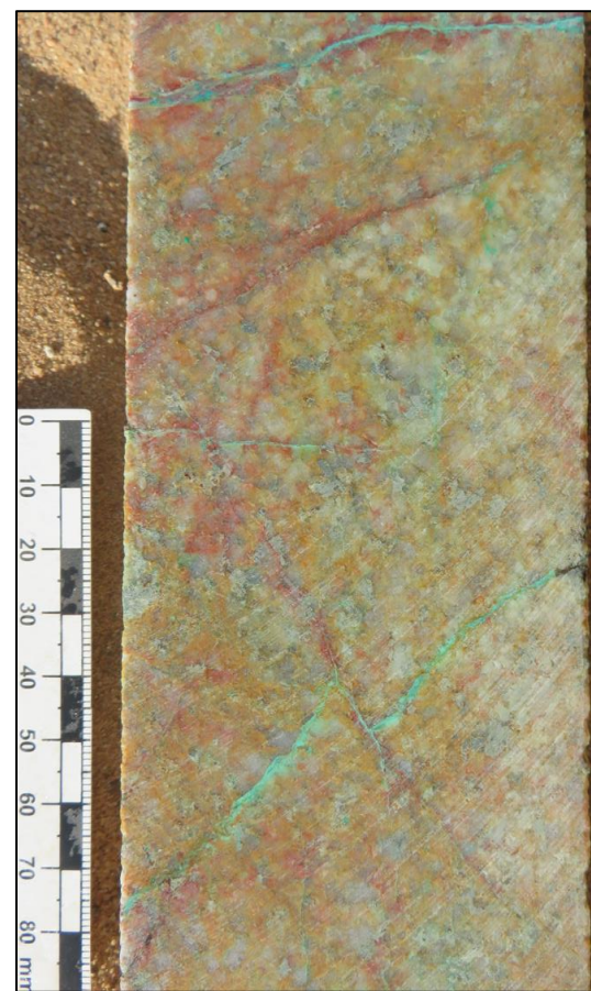
Secondary Cu-Ox in veinlets within ferruginous, phyllic-altered granite in CDDH-013 (13.5m)
